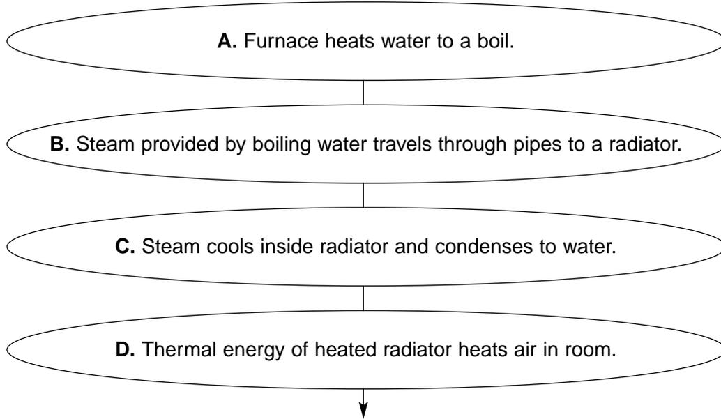
1. Is the system in the flowchart a hot-water system or a steam-heating system?
