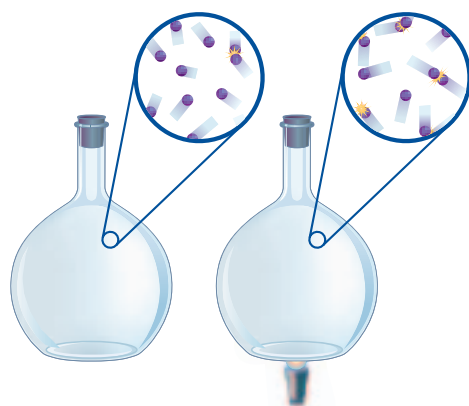
Figure 21 Even though the volume of this container does not change, the pressure increases as the substance is heated.
