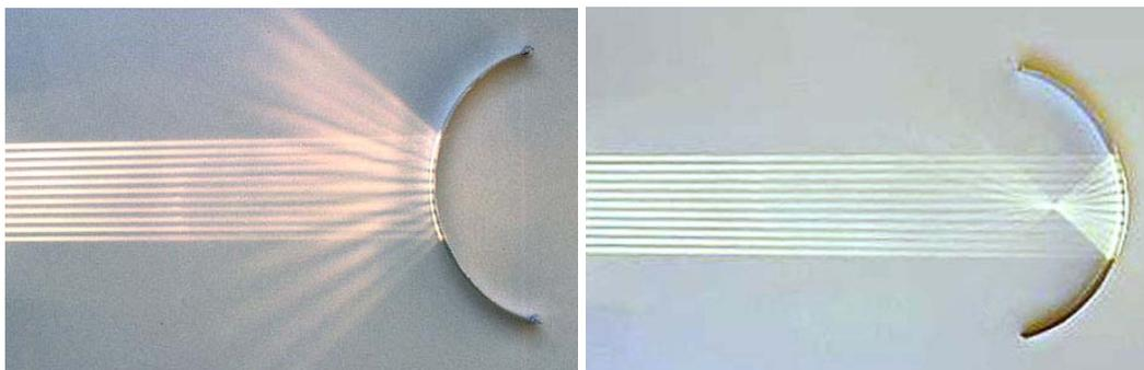
*Figure 8: Reflection from a convex mirror (left) and from a concave mirror (right). For each light ray we can apply the rule that angle of incidence is the angle of reflection. These angles are measured from a line perpendicular to the surface of the mirror (the normal line). However at every point this perpendicular line has a different orientation.*
