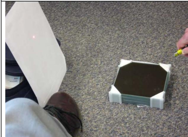
*Figure 3a Mirror reflection: The laser pointer is directed at the mirror. However, looking from the side we do not see a lighted spot on the mirror. All the laser light is reflected in one direction only, towards the white paper screen. On the screen we see a light spot as the screen reflects the light diffusely to all directions including the direction of the camera*
