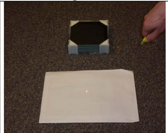
*Figure 3b Diffuse reflection: The laser pointer is directed towards the white paper screen. From there the light is reflected in all directions including the direction of the camera. So the light spot is visible from all sides.*
