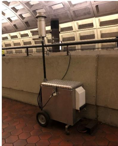
**Figure 7: BioWatch air-monitoring device**
