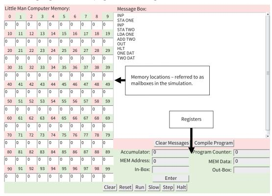
Before the program can be run, it must be compiled into machine code.
