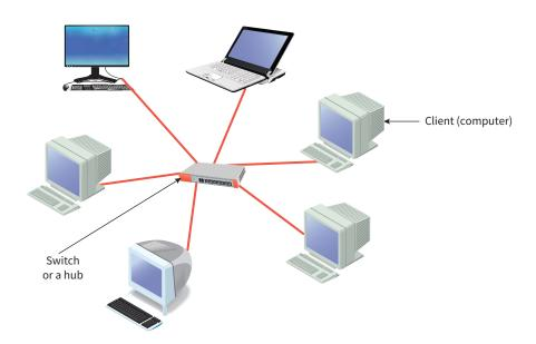
Using a star topology, each computer is connected individually to a central point, which can be a file server or switch. The computers are individually connected by cable to a switch. The cable is connected to the network adapter in each device.
