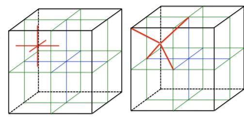
of <u>one</u> of these holes is shown two different ways in the figures below. The Cartesian coordinates shown in the figure on the left only indicate the center of the tetrahedral hole. How many tetrahedral holes are present within a fcc unit cell?
